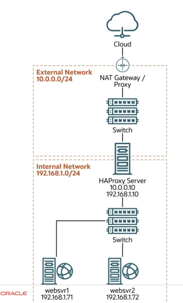
Figure 2-1 Example HAProxy Configuration for Load Balancing
