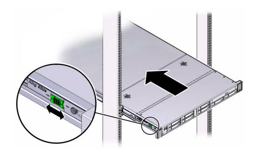
b. Continue pushing the server into the rack until the slide-rail locks (on the front of the server) engage the slide-rail assemblies.
