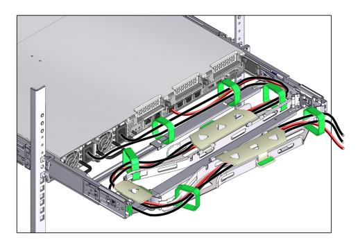
16. Ensure that the secured cables do not extend above the top or below the bottom of the server to which they are attached, otherwise, the cables might snag on other equipment installed in the rack when the server is extended from the rack or returned to the rack.
