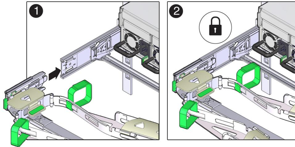
9. Gently tug on the left side of the CMA's slide bar to verify that connector D is properly seated.
