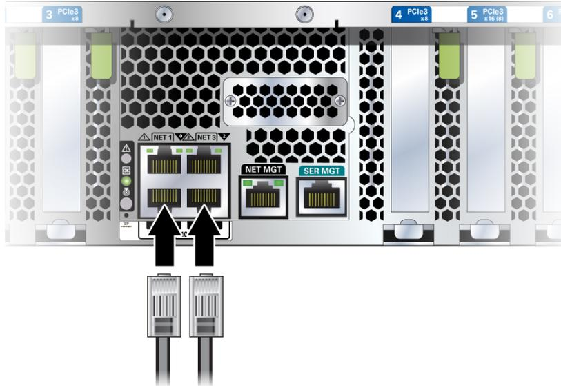
2. Connect Category 5 (or better) cables from your network switch or hub to the remaining Ethernet ports (NET 1, NET 2, and NET 3), as needed.
