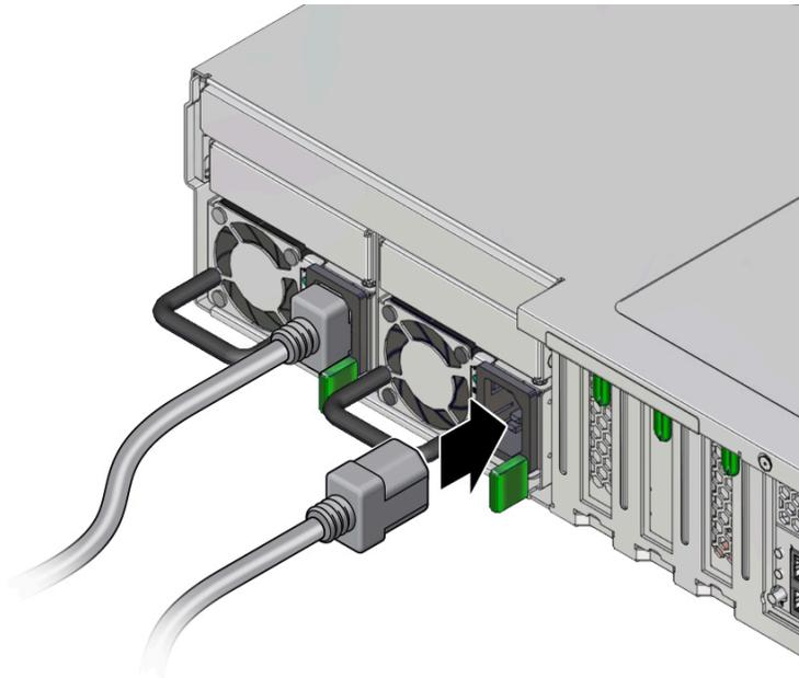
When the power cords are connected, the SP initializes and the power supply LEDs illuminate. After a few minutes, the SP login prompt is displayed on the terminal device. At this time, the host is not initialized or powered on.
