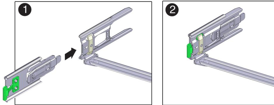
**8. Install the CMA's connector D into the left slide rail.**
