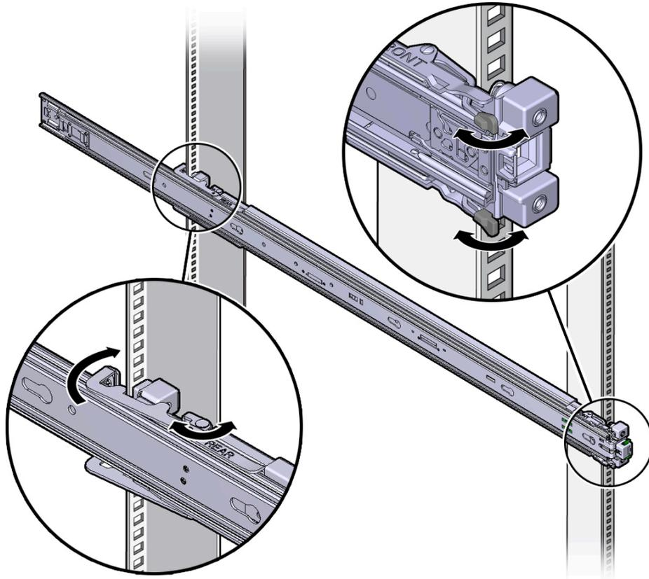
8. Align the front of the slide rail assembly against the outside of the front rack rail, and push until the assembly locks into place with an audible click.
