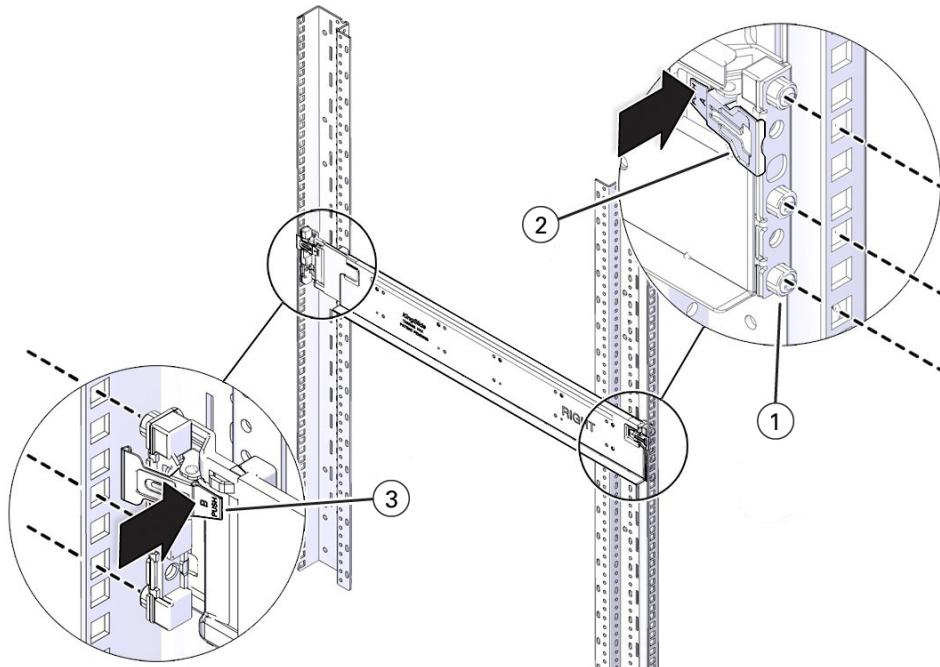
**6. Attach the back mounting brackets.**
