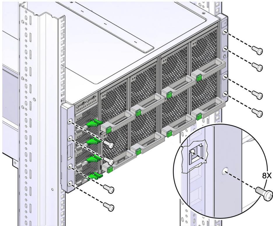
4. **Press the back mounting brackets against the server and tighten the screws.**
