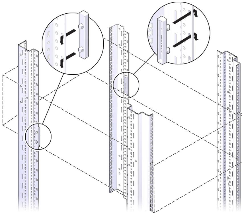
**4. Use the alignment template to install cage nuts.****a. Align the template with the holes where you intend to place the server.**
