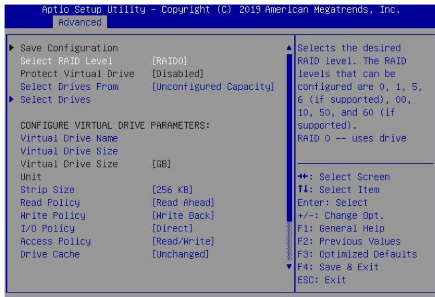
7. Set the RAID level. Choose **Select RAID level**, specify the supported RAID level, and press **Enter**.
