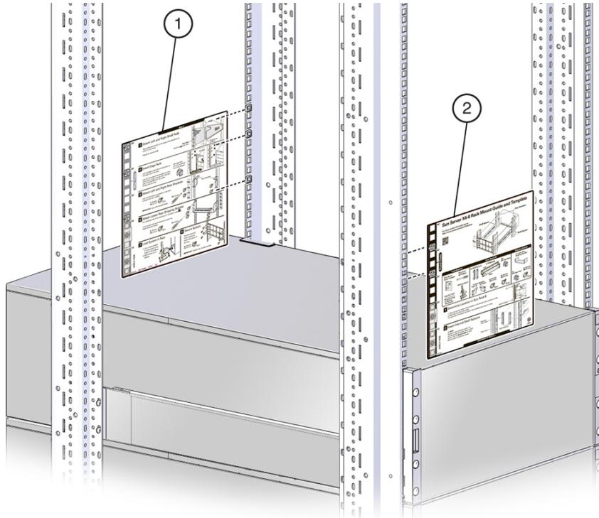
**b. Place the cage nuts in the locations indicated by the rack alignment template.**
