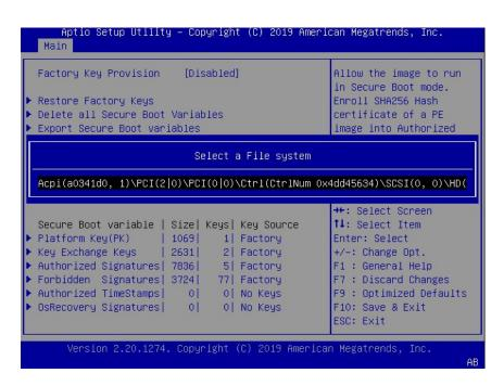
a. On the Select a File System screen, Scroll through the list and select the file system that contains the EFI file and press Enter.
