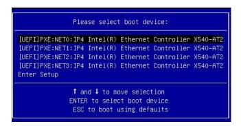
3. In the Please Select Boot Device dialog box, select the boot device according to the operating system you elected to use, and then press Enter.
