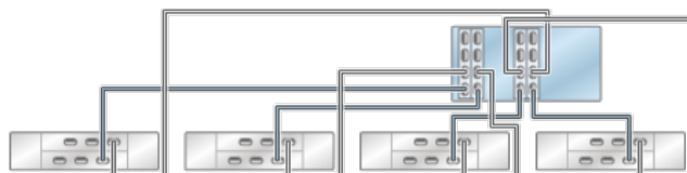
Standalone Sun ZFS Storage 7420 controller with four HBAs connected to four Oracle Storage Drive Enclosure DE2-24 disk shelves in four chains
