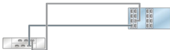
Standalone Sun ZFS Storage 7420 controller with four HBAs connected to two Oracle Storage Drive Enclosure DE2-24 disk shelves in two chains
