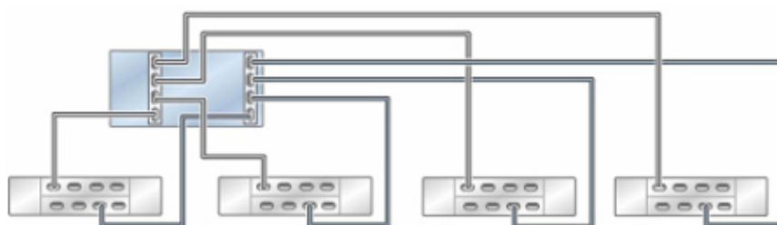
Standalone Oracle ZFS Storage ZS9-2 MR controller with two HBAs connected to four Oracle Storage Drive Enclosure DE3-24 disk shelves in four chains
