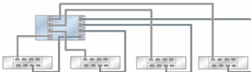
Standalone Oracle ZFS Storage ZS7-2 MR controller with two HBAs connected to four Oracle Storage Drive Enclosure DE3-24 disk shelves in four chains
