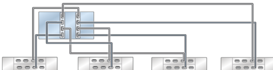
Standalone Oracle ZFS Storage ZS4-4 controller with two HBAs connected to four Oracle Storage Drive Enclosure DE3-24 disk shelves in four chains
