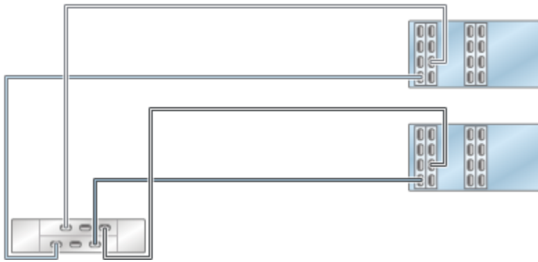
Clustered Sun ZFS Storage 7420 controllers with four HBAs connected to two Oracle Storage Drive Enclosure DE2-24 disk shelves in two chains
