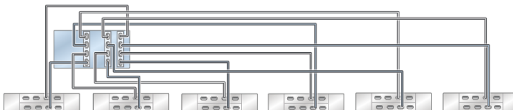
Standalone Oracle ZFS Storage ZS4-4 controller with three HBAs connected to six Oracle Storage Drive Enclosure DE3-24 disk shelves in six chains
