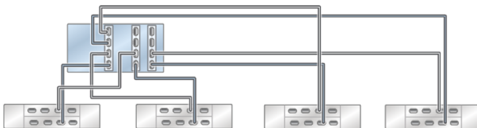
Standalone Oracle ZFS Storage ZS4-4 controller with three HBAs connected to four Oracle Storage Drive Enclosure DE3-24 disk shelves in four chains
