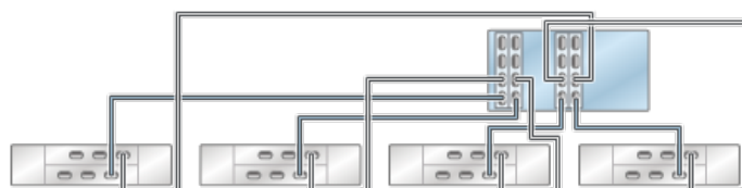
Standalone Oracle ZFS Storage ZS4-4/ZS3-4 controller with four HBAs connected to four Oracle Storage Drive Enclosure DE2-24 disk shelves in four chains
