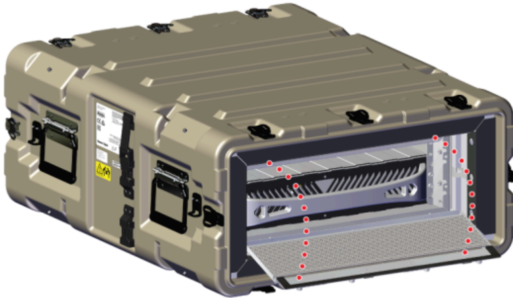
Figure 14: Rotating and Seating the Front EMI Filter Assembly
