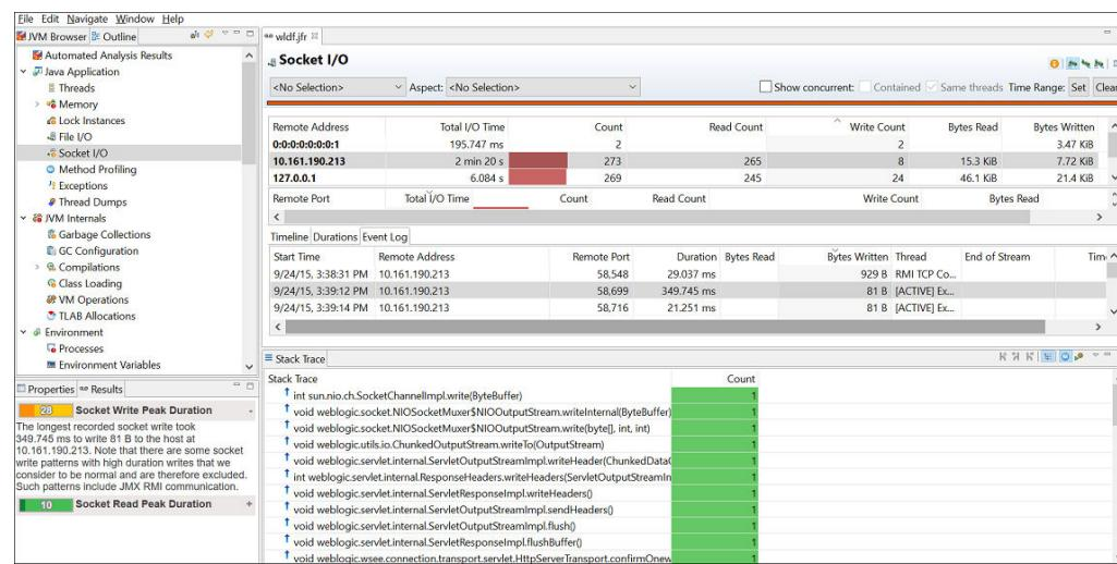
The figure shows that for the application the longest recorded socket write took 349.745 ms to write 81 B to the host.
