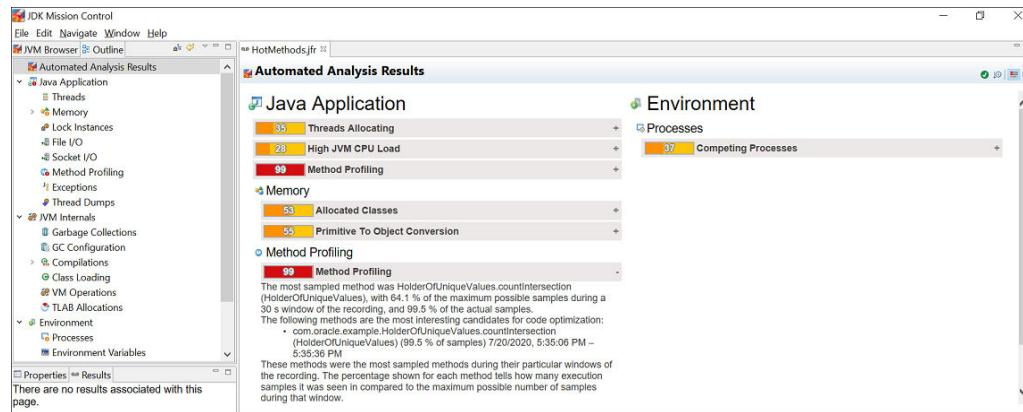
Now, open the **Java Application** page. Here is a sample figure of a recording, which shows the **Method Profiling** graph and the stack traces.
