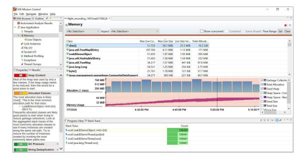
You can observe from the graph that the memory usage has increased steadily, which indicates a memory leak issue.
