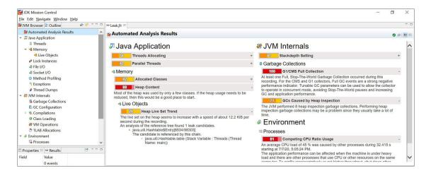
You can observe that in the **Heap Live Set Trend** section, the live set on the heap seems to increase rapidly and the analysis of the reference tree detected a leak candidate.
