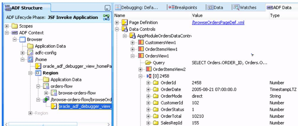
Expanding the Parameters node in the ADF Data window displays information similar to that shown in Figure 31-42.
