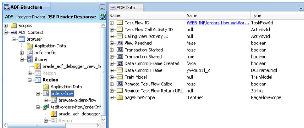
The roots of the hierarchy are the sibling nodes **Scopes** and **ADF Context**. The current view port where processing has stopped appears in bold. Default selections within the tree will be retained from the previous breakpoint, so you can monitor any changes between breakpoints. The ADF object where the ADF declarative breakpoint was defined will be opened in the corresponding JDeveloper editor, either the task flow diagrammer or the overview editor for page definition files.
