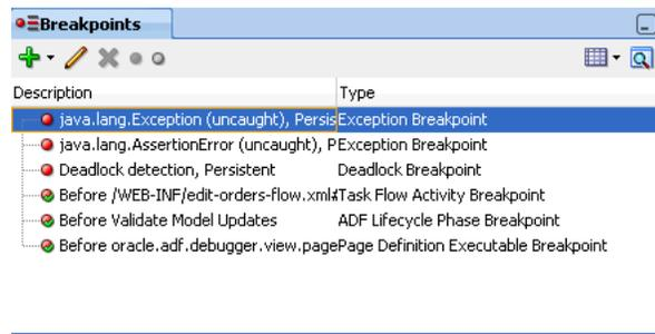
When an ADF declarative breakpoint is set, it appears as a red dot icon in the task flow activity, in the page definition breakpoint margins, or in the ADF Lifecycle Breakpoints window, as shown in [Figure 31–22](#), [Figure 31–23](#), and [Figure 31–24](#).
