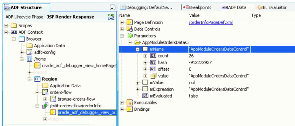
Expanding the Executables node in the ADF Data window displays information similar to that shown in Figure 31-43.
