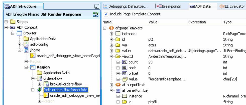
When you select a binding container in the ADF Structure hierarchy, it displays within the ADF Data window the node selection listed in [Table 31–8](#).
