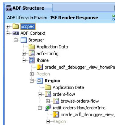
When you select an item in the ADF Structure window, the data and values associated with that item are displayed in the ADF Data window. [Figure 31–33](#) shows a task flow
