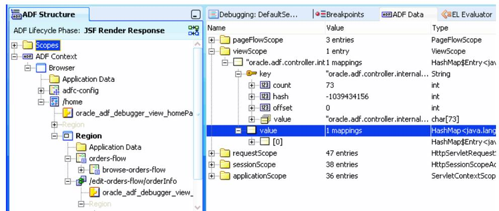
When the ADF context is selected in the ADF Structure window, as shown in Figure 31–36, the current value of the ADF context variables will be displayed in the ADF Data window. You can also inspect ADF context variables and values by evaluating the # (data.adfContext) EL expression in the EL Evaluator. For more information, see Section 31.7.4, "How to Use the EL Expression Evaluator."
