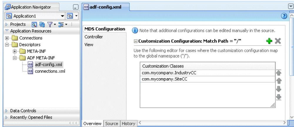
The order of the customization-class elements defines the precedence of customization layers. For example, in the code shown in Example 34–6, the `IndustryCC` class is listed before the `SiteCC` class. This means that customizations at the industry layer are applied to the base application, and then customizations at the site layer are applied.
