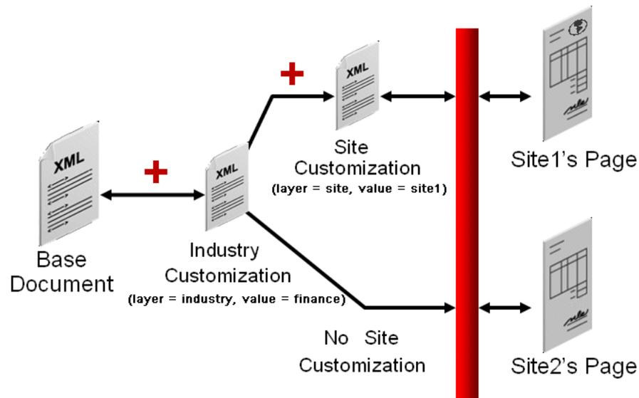
To support this, you use JDeveloper to create customization classes, define layers and values, and specify the order of precedence. These processes are described in [Section 34.2, "Developing a Customizable Application."](#)
