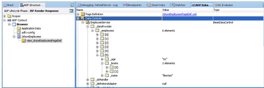
When you select a binding container for an application based on ADF Business Components objects, the ADF Data window displays standard row collection icons, as shown in Figure 31-2.
