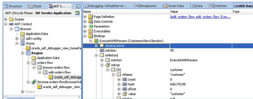
When you select an Application Data node from the ADF Structure window, the ADF Data window displays the application objects, such as ADF Business Components objects, instantiated within the current data control frame for the corresponding view port (or binding context if ADF Controller is not used).
