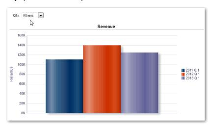
The graph is the detail view, with the City prompt listening for events from the table view on the specified CityChoice channel. Suppose the user clicks on a value in the City column in the table view. The, prompt in the graph view is set to that city, and the graph is refreshed.
