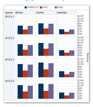
The trellis view, also referred to as a trellis graph, is the same as a pivot table—with one major exception: the data cells within the trellis contain graphs. Whereas a stand-alone graph type such as a single bar graph or a single scatter graph works on its own, the trellis graph works only by displaying a grid of nested graphs, known as inner graphs. So a bar-graph trellis view is actually comprised of multiple bar graphs.
