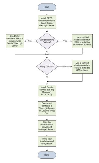
Figure 1–1 Oracle Service Bus Install Flow for a Development Environment
