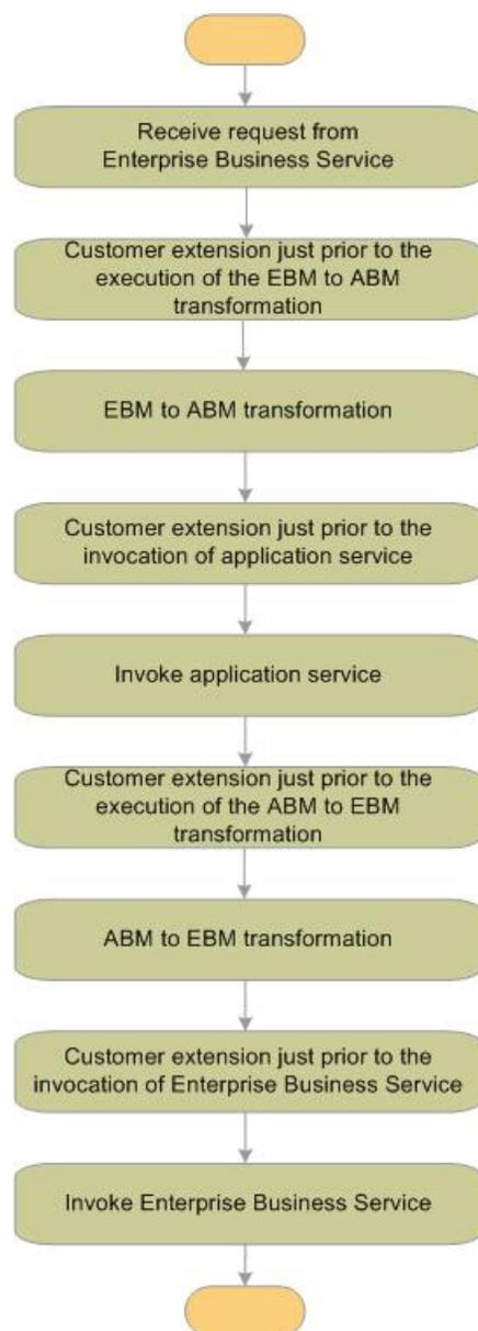
Figure 4–5 depicts the high-level flow of activities in a provider-specific ABCS. The EBS and ABCS interact in a fire-and-forget style.
