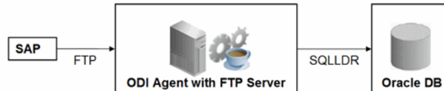
Figure 7-3 Configuration 1: FTP Server is installed on an ODI Agent machine
