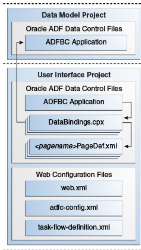
Figure 3–6 depicts the connection between the data controls, declarative bindings, and view layer.
