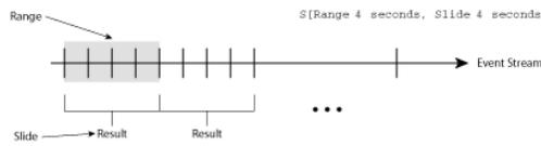
In [Figure 1-4](#), the Range specification indicates "I want to look at 8 seconds worth of data" and the Slide specification indicates "I want a result every 4 seconds". In this case, the query returns a result twice during each Range specification (except for certain conditions, as [Range, Rows, and Slide at Query Start-Up and for Empty Relations](#) describes)
