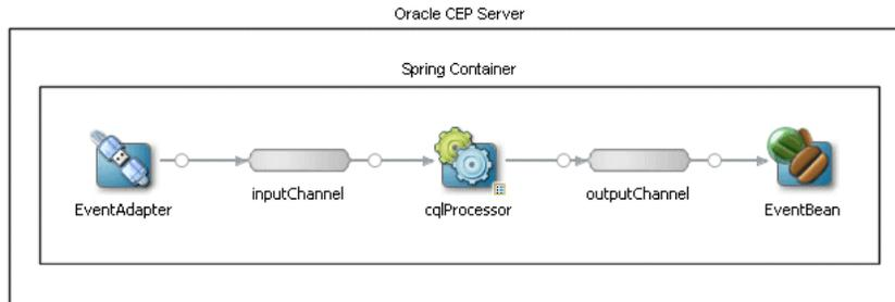
Using Oracle Event Processing, you can define event adapters for a variety of data sources including JMS, relational database tables, and files in the local filesystem. You can connect multiple input channels to an Oracle CQL processor and you can connect an Oracle CQL processor to multiple output channels. You can connect an output channel to another Oracle CQL processor, to an adapter, to a cache, or an event Bean.
