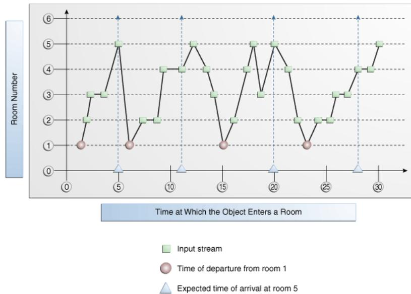
The following example shows query `q` on stream `S` (with schema `c1 integer` representing room number) that detects these non-events. Each time the object fails to reach room 5 within 5 minutes of leaving room 1, the query returns the time of departure from room 1.
