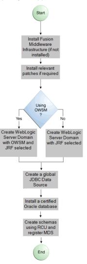
Figure 4-1 Preparing the Application Server Flow Diagram
