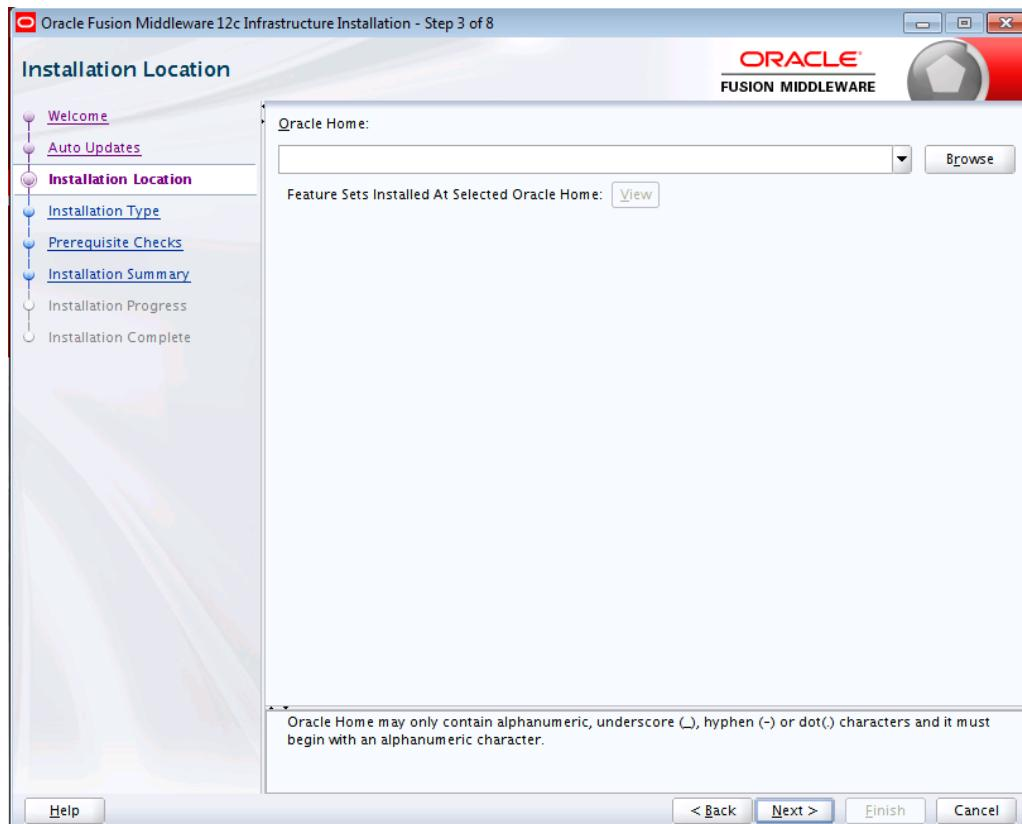
If you have an existing directory into which one or more Oracle products have already been installed, that directory can be viewed in the drop-down list. You can see which products are installed in that particular directory by clicking **View** next to "Features Sets Installed At Selected Oracle Home."
