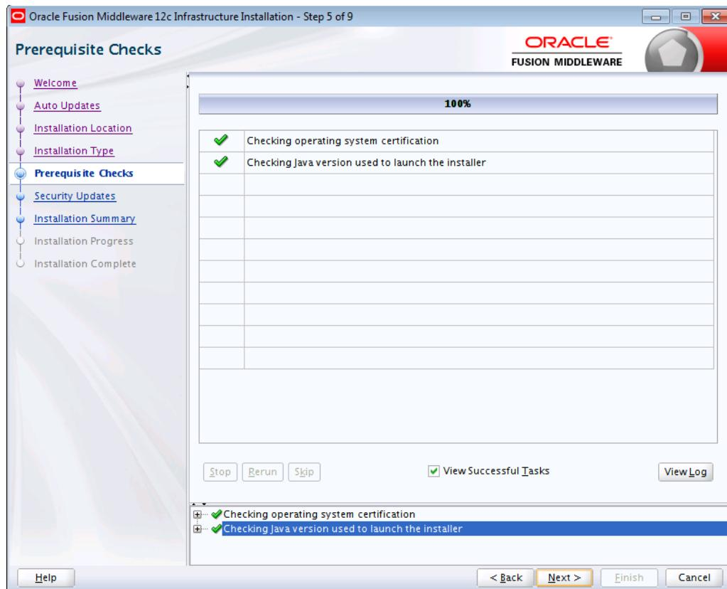
This screen analyzes the host computer to ensure that specific operating system prerequisites have been met.
