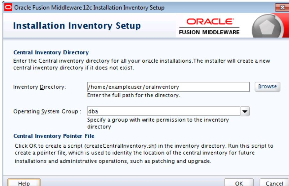
If this is your first Oracle installation on a host that is running UNIX or Linux system software, you must use this screen to specify the location of the Oracle central inventory directory.
