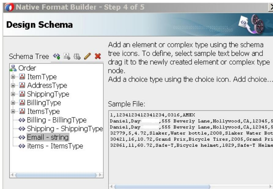
When complete, a schema file is created. [Figure 5-6](#) provides details.
