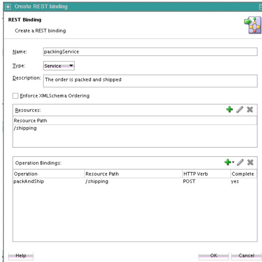
This creates a REST service binding component in the **Exposed Services** swimlane, as shown in [Figure 6-5](#).
