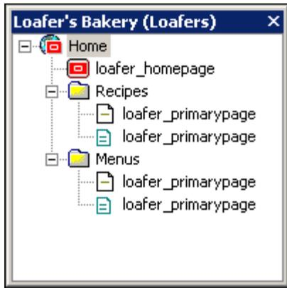
The same page template was used for both the primary and secondary pages. The page template name was based on where the template was based on initial placement, and when the site was expanded the reuse of the page template created a confusing arrangement.
