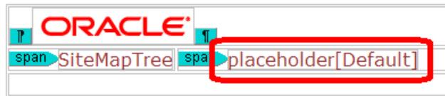
Placeholder marker in design view, with table layout being used for positioning objects on the page. The image shows a three-row table, with an image in the top row, a SiteMapTree fragment and a marker for a placeholder called "Default" in the second row, and a blank third row.
