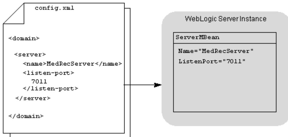
The configuration MBeans enable each server instance in the domain to have an identical in-memory representation of the domain's configuration.
