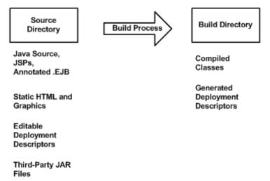
The build directory contains only those files generated during the build process. The combination of files in the source and build directories form a deployable Java EE application.
