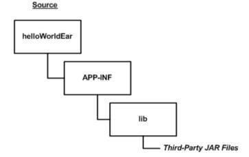
Third-party JARs are generally not compiled, but may be versioned using the source control system for your application code. For example, XML parsers, logging implementations, and Web application framework JAR files are commonly used in applications and maintained along with editable source code.
