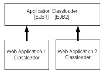
This hierarchy is optimal for most applications, because it allows call-by-reference semantics when you invoke EJBs. It also allows Web modules to be independently reloaded without affecting other modules. Further, it allows code running in one of the Web modules to load classes from any of the EJB modules. This is convenient, as it can prevent a Web module from including the interfaces for EJBs that it uses. Note that some of those benefits are not strictly Java EE-compliant.
