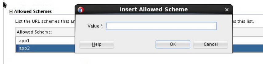
Figure 3-1 Registering a Custom URL Scheme that a MAF Applications Use to Invoke Another Application
