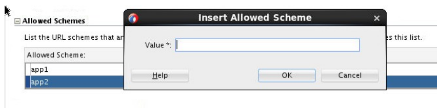
Figure 5-2 Registering a Custom URL Scheme that a MAF Applications Use to Invoke Another Application
